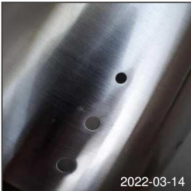
Where and tear on the top of the lamp
